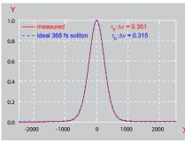
X TIME DELAY (fs) Y AUTOCORRELATION SIGNAL
